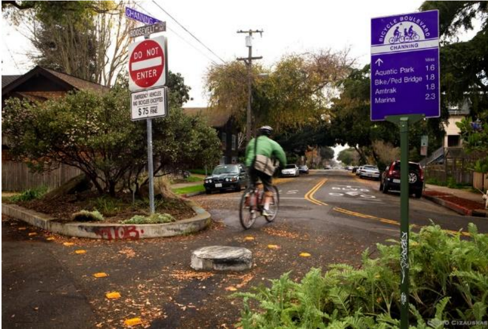
Figure 12. Bike boulevards include shared lanes on a low-volume, low speed street with bike and pedestrian prioritization features.
