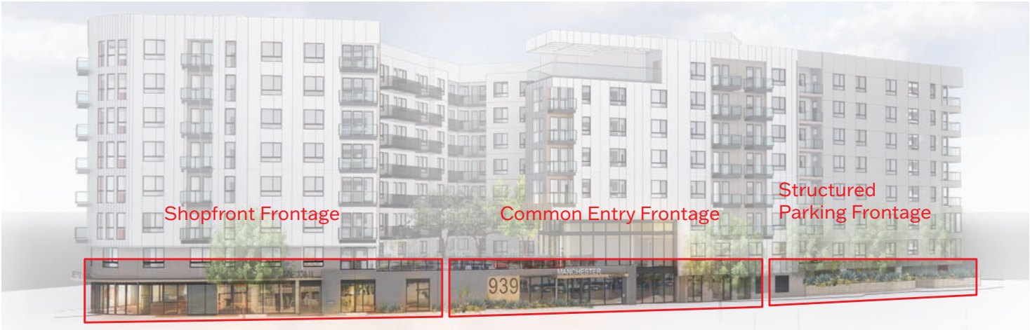
4.1: Example of the diagram each applicant shall submit indicating which frontage types are being used in different portions of each building.
